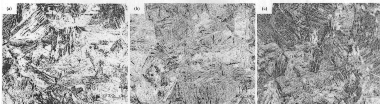
图4 Q235 钢奥氏体组织形貌 \times 500 :淬火温度-(a) 950 °C; (b) 1000 °C; (c) 1050 °C Fig. 4 Morphology of structure of austenite in steel Q235, \times 500 : quenching at (a) 950 °C; (b) 1000 °C; (c) 1050 °C
